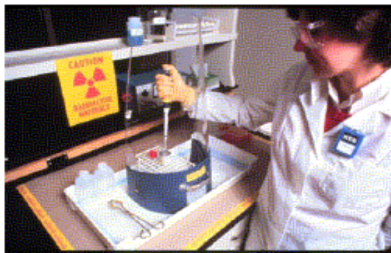
Figure 18 Use of Plexiglas Shielding
