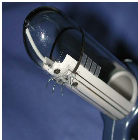
Fig. 6. Four titanium needle electrodes in the operating head of the handpiece. From Efron JE, Corman ML, Fleshman J, et al. Safety and effectiveness of temperature-controlled radio-frequency energy delivery to the anal canal (Secca procedure) for the treatment of fecal incontinence. Dis Colon Rectum 2003;46(12):1606–18; with permission.
