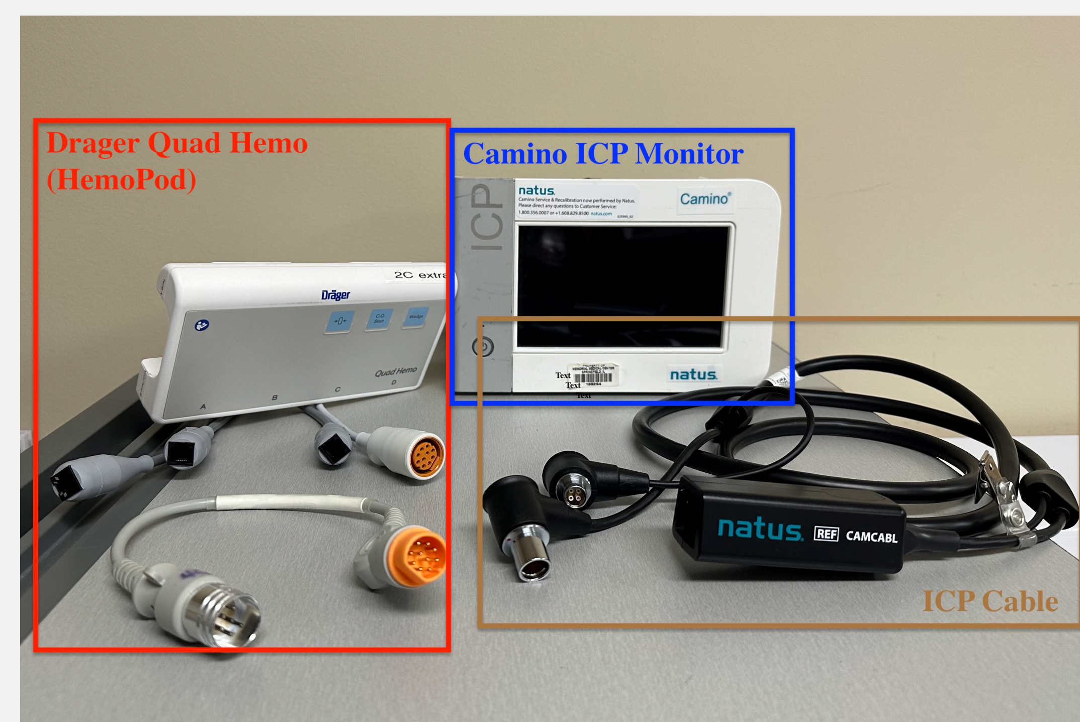
Figure 4. Nursing supplies for Camino ICP monitoring. Drager Quad Hemo or HemoPod (Red); Camino ICP monitor (Blue); ICP Cable (Brown)
